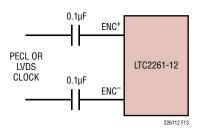
Figure 13. PECL or LVDS Encode Drive
