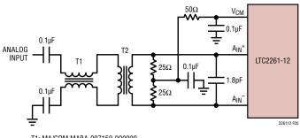
T1: MA/COM MABA-007159-000000 T2: COILCRAFT WBC1-1LB RESISTORS, CAPACITORS ARE 0402 PACKAGE SIZE
