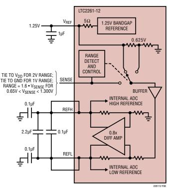
Figure 8. Reference Circuit
