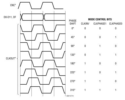
Figure 14. Phase Shifting CLKOUT
