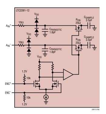
Figure 2. Equivalent Input Circuit
