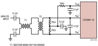
T2: MA/COM MABAES0060 RESISTORS, CAPACITORS ARE 0402 PACKAGE SIZE
